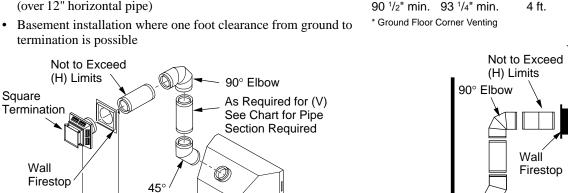
Figure 15 - Horizontal Termination Configuration for Corner Installation Using One 90° Elbow
